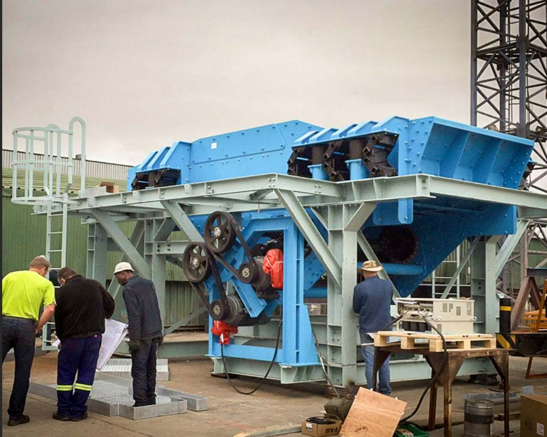
6200X2280 SCALPING GRIZZLY CUTTING AT 150MM
